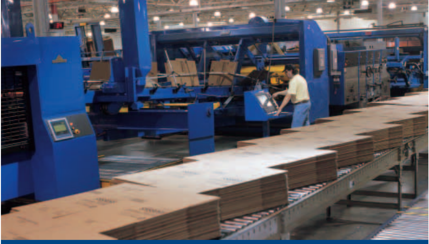
PCA's new 50" flexo folder/gluer at our Milwaukee, Wisconsin facility has increased production flow.
