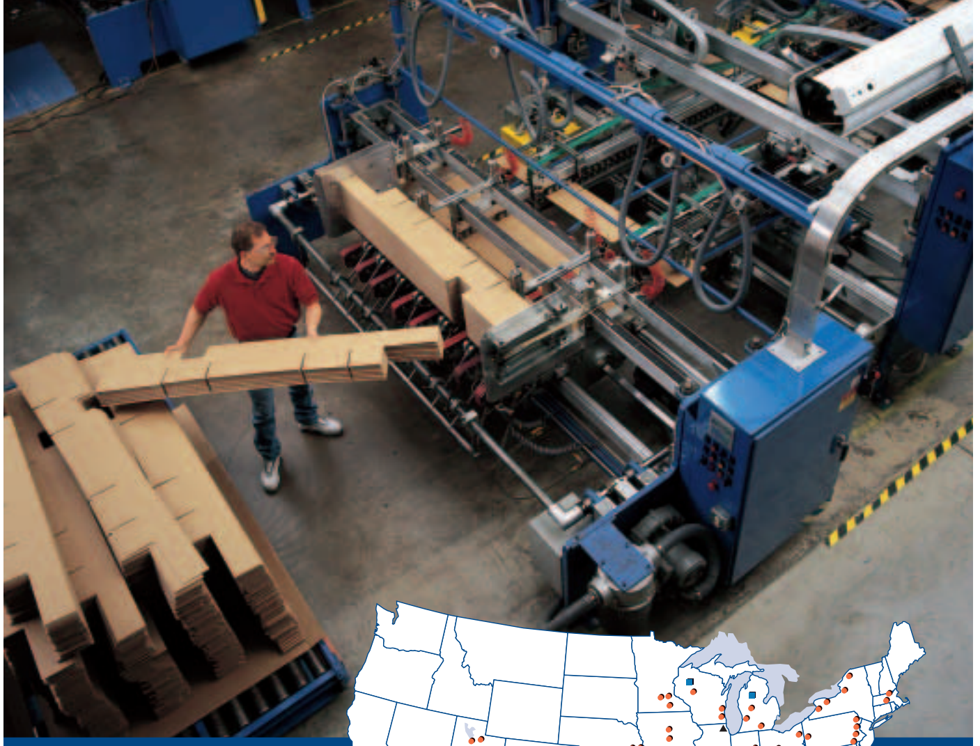
This specialty folder/gluer at our Burlington, Wisconsin facility is used to glue various styles of corrugated containers and display components.
